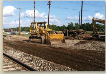
A key component of Hulcher Services' derailment response service is the Caterpillar® 977 / 973 track loader.
