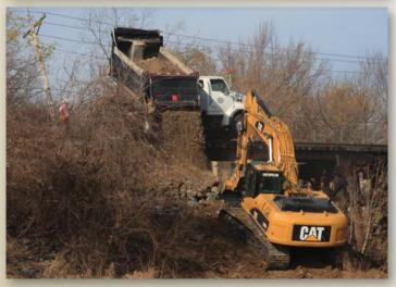
Hulcher Services' hi-rail rotary dump truck is designed specifically for railroad work.
